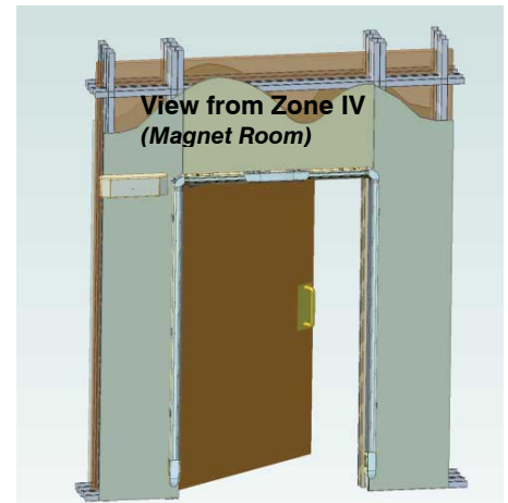
Figure 6: SuiteSentry mounted IN side MR; OUT swing Door
