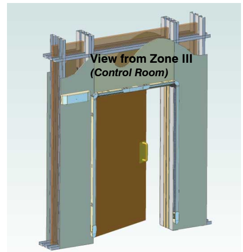
Figure 5: SuiteSentry mounted OUT side MR; IN swing Door
