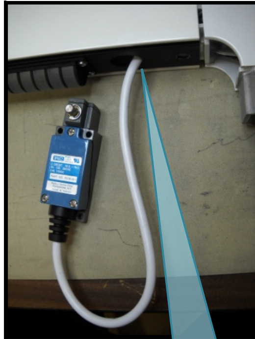
Figure 26: Cable extended to mount switch externally
