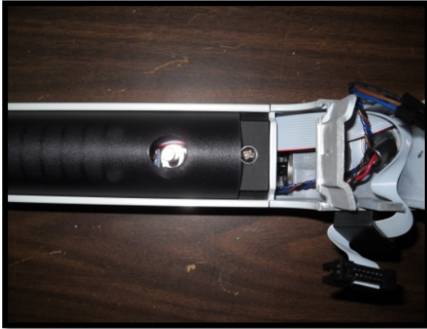
Figure 25: Switch mounted in crossbar
